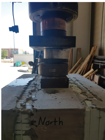
Spherical bearing and load cell sandwich
