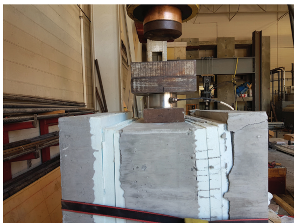
Load cell sandwich without spherical bearing
